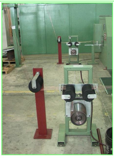
The capstan is a device that, put in line with wire and cables during the unwinding, allows to equalize the tensions on products. The braking system is "disk separation" type with adjustable pneumatic reaction. This system guarantees a constant braking and a a game of cushioning during starting and braking ramps of the line. The braking element has a very long duration.
